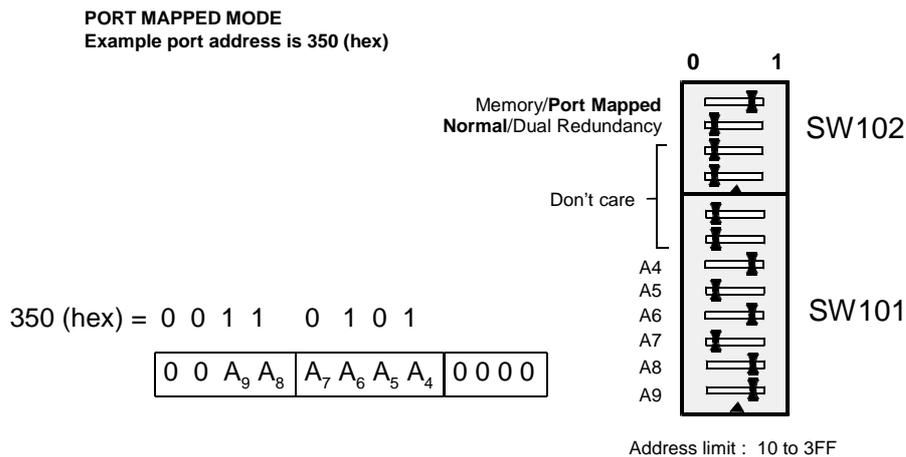
**Figure 2.8** Port mapped mode: switch setup example.
