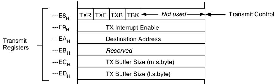
**Figure 4.6 Transmit registers.**
