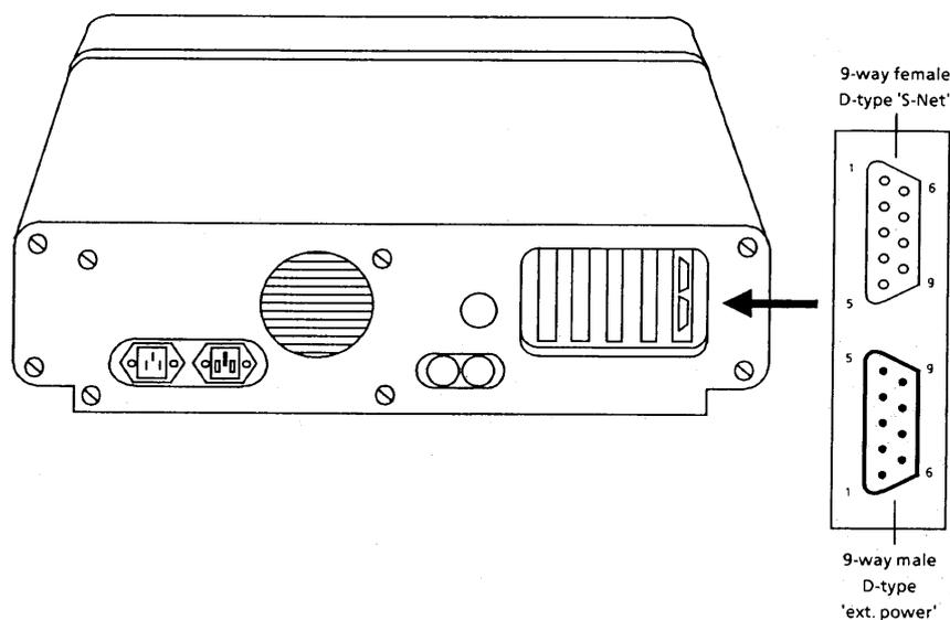
**Figure 2.17** Location of the 'ext power' connector on the PC rear panel.
