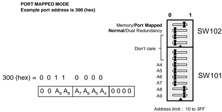
**Figure 2.7** Port mapped mode: switch setup example 1
