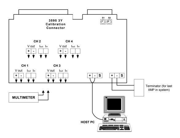
Figure 1.4: Connections to '3595 3Y' calibration block connector
