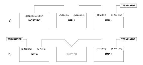
Figure 2.1: S-Net cable terminations
