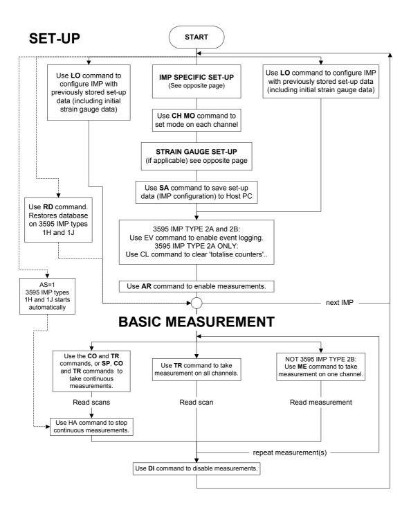
Figure 1.5: Set-up and basic measurement
