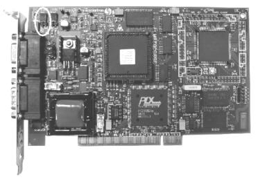
Figure 2.3: Location of external power supply Jumper J201
