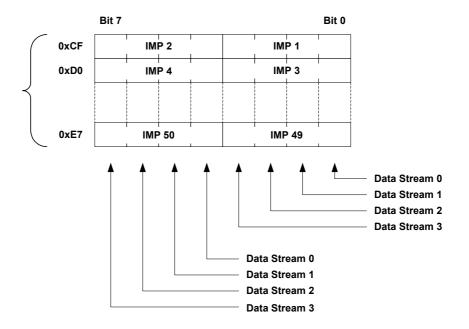
Figure 3.7: Receive Interrupt Table
