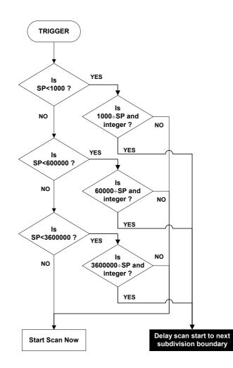
Figure 1.2: Scan synchronisation of 1H and 1J IMP types
