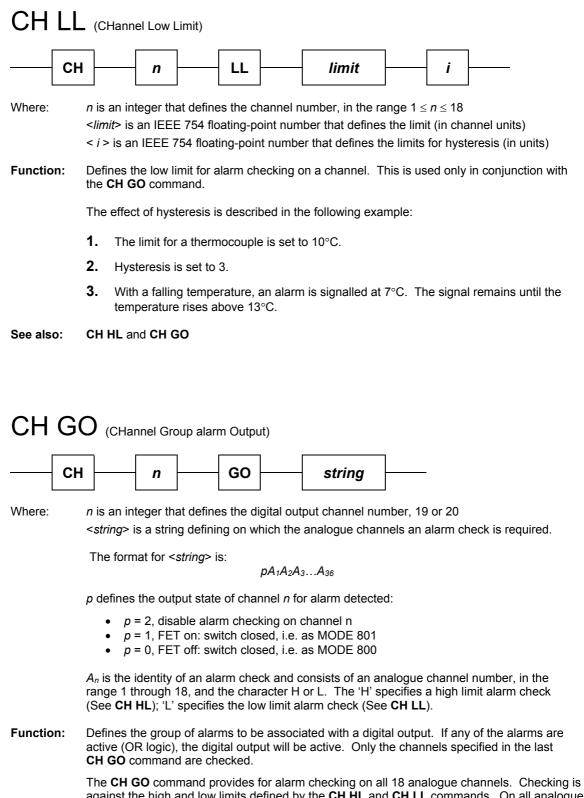
The CH GO command provides for alarm checking on all 18 analogue channels. Checking is against the high and low limits defined by the CH HL and CH LL commands. On all analogue channels, it is possible to specify a high limit alarm check, or a low limit alarm check, or both. Specifying both alarm limit checks is equivalent to specifying an 'out-of-window' check. (Note that it is not possible to specify an 'in-window' check by specifying a high limit that is less than the low limit.)
