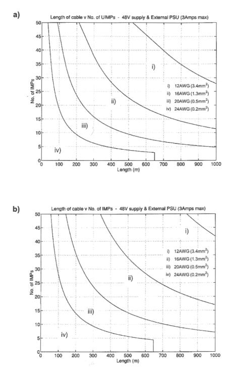
Figure 2.8: Minimum recommended wire gauge for a 48V external supply for: (a) Universal IMP and (b) Other IMP
