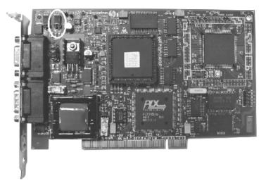
Figure 2.2: Location of S-Net termination Jumper J202
