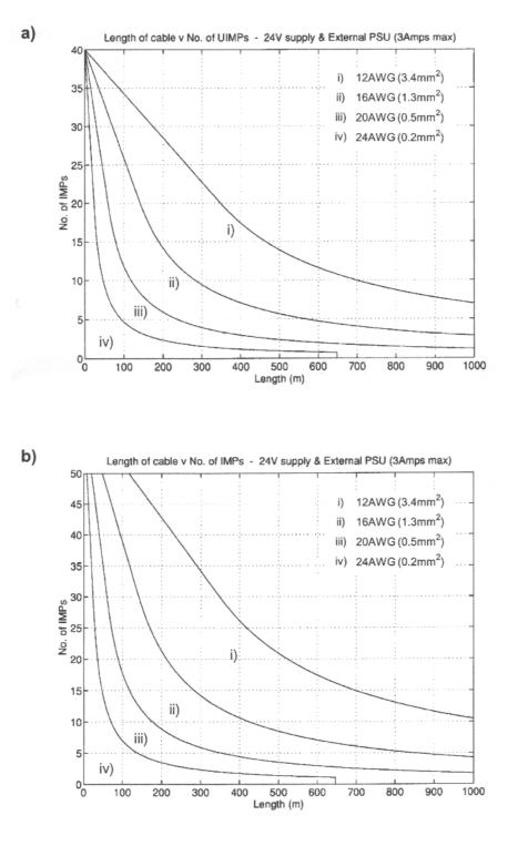
Figure 2.7: Minimum recommended wire gauge for a 24V external supply for: (a) Universal IMP and (b) Other IMP
