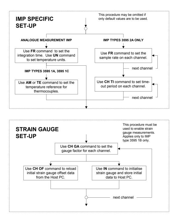
Figure 1.6: IMP Specific Set-up and Strain Gauge Set-up
