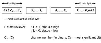
**Note:** Channel numbers entered for the 3595 2A IMP correspond exactly with the physical channels: 1 = Channel 1, 2 = Channel 2, etc. With the 3595 2B IMP, however, channel numbers 0 through 31 represent the physical channels 1 through 32.
